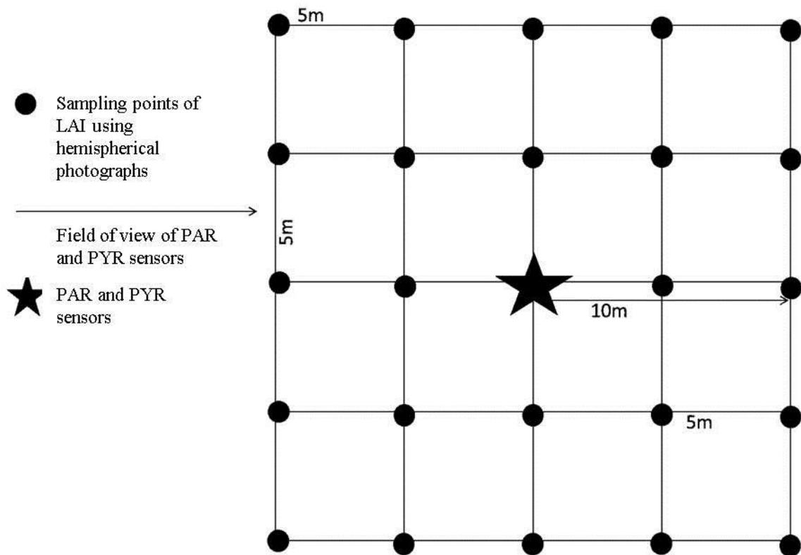
Figure 1. Sampling points of LAI within the field-of-view limit (10 m) of PAR and PYR sensors.
